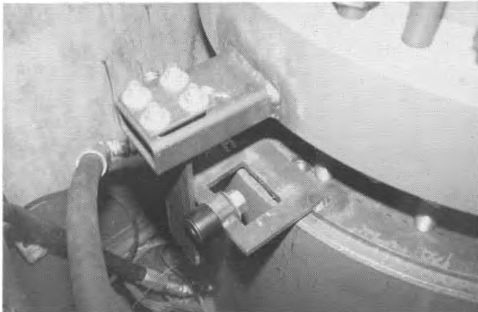
Figure 5.7 Rotation restraint device
