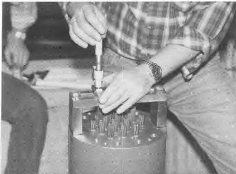
Figure 5.4. Measurement of center wire and wedge seating with a depth gage and stationary fixture
