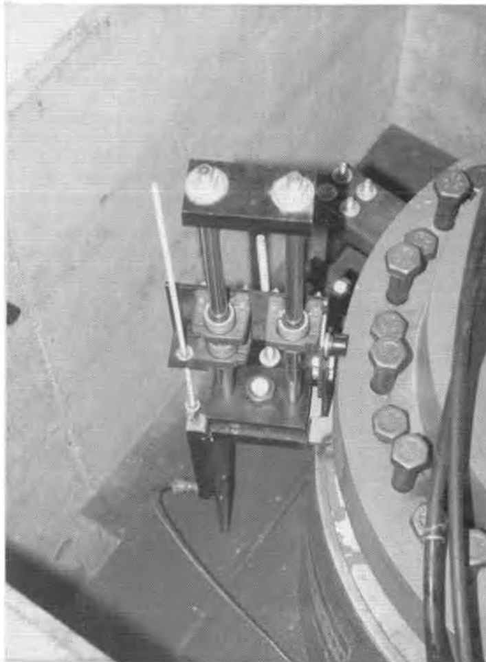
Figure 5.5 Linear potentiometer to measure specimen elongation
