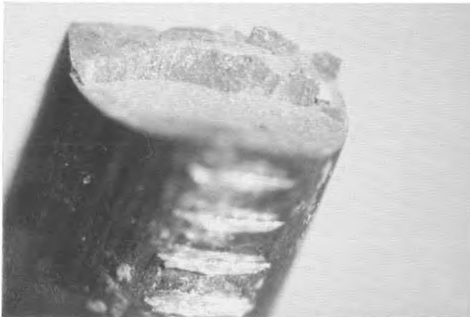
Figure 5.35 Outer wire failure in wedges of top anchorhead, strand 18
