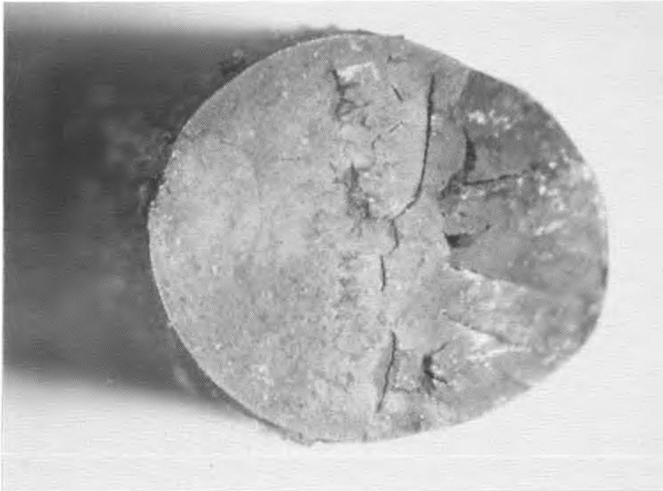
Figure 5.32 Outer wire failure in wedges of top anchorhead, strand 10
